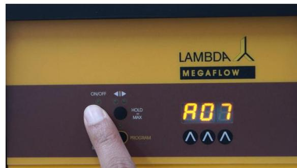
**Figure 4-6** To confirm the address and save it, press the **ON/OFF** button.
