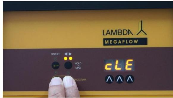
**Figure 2-2** Continuous pressing of **REMOTE** and **RUN** button even after the indication of “**PGM**” ends up with the “**cLE**” indication.
