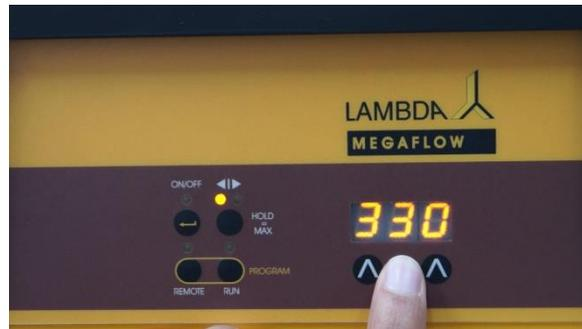
**Figure 2-4** Set the desired flow rate value for the first program step by pressing the buttons ▲▲▲ below the display (from 0 to 999, corresponding to 0 to 100% of the motor rotation speed).
