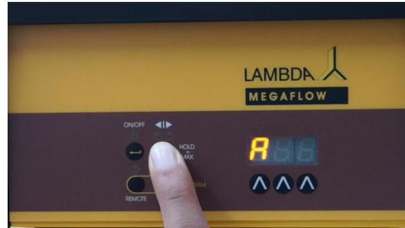
**Figure 4-4** The message “A” and two numbers will appear on the display. This number from 00 to 99 is the current address of the pump.
