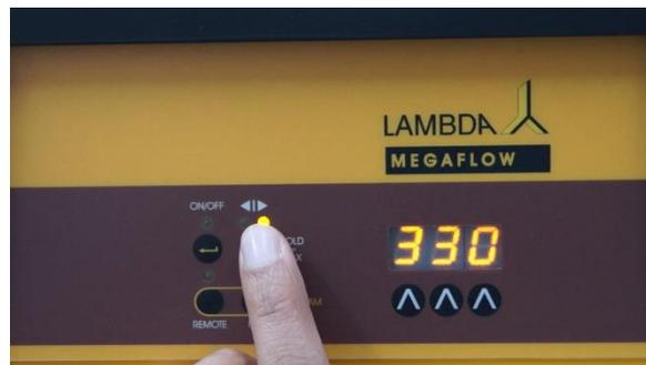
**Figure 1-6** LED illumination in the direction |▶ represents the anticlockwise rotation.
