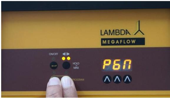
**Figure 2-1** Press the **REMOTE** and **RUN** simultaneously until the indication “**PGM**” appears on the display.
