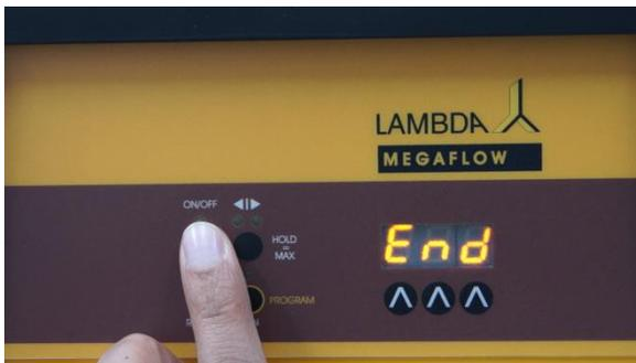
**Figure 2-19** Press the **ON/OFF** button until the indication “End” appears on the display to confirm and save the program.
