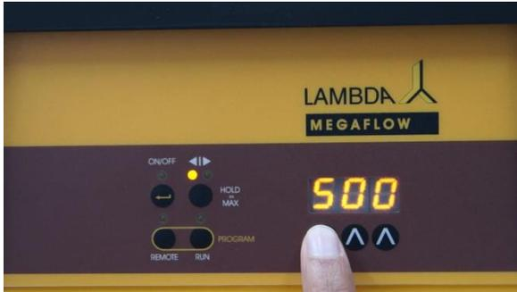
**Figure 1-3** The ▲▲▲ buttons can be used to set the desired flow rate.
