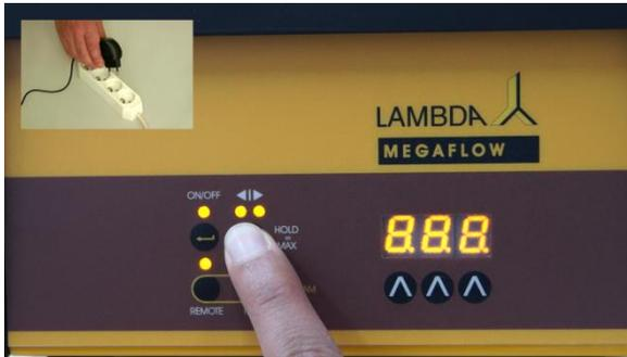
**Figure 4-3** Disconnect the pump from the mains. While keeping the direction button ◀▶ pressed, connect the pump to the mains again.
