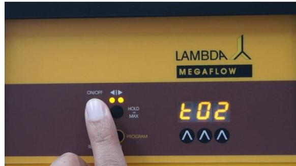
**Figure 2-12** Press the ON/OFF button again, the symbol “t02” will briefly appear on the display.
