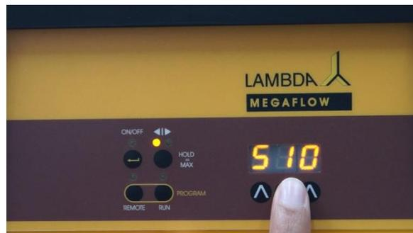
**Figure 2-10** Enter the desired flow rate for the second program step.
