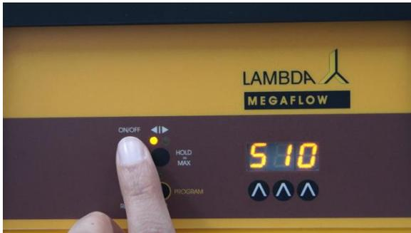
**Figure 2-11** If the ◀ button is not used to change the direction, the default pump rotation for the set speed is clockwise, ◀ LED ON.
