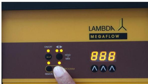
**Figure 1-7** Plug-in the power supply and at the same time press the **RUN** button on the control panel.
