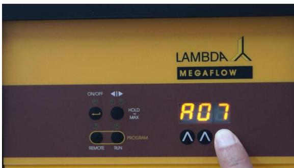
**Figure 4-5** To change the address press the buttons ▲ ▲ ▲ under the display until the desired number is obtained.
