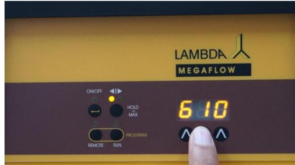
**Figure 1-4** Each ▲▲▲ arrow can be used to change the corresponding digit on the flow rate.
