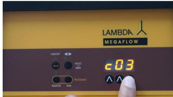
**Figure 2-18** If you wish to repeat the same program 3 times, increase the cycle number to “c03” by pressing the buttons  $\wedge \wedge \wedge$  below the display (from 0 to 99 cycles). The program can be repeated up to 99 times, indicated by “c99”. If 0 is entered for the cycle number “c00”, the program will run continuously (infinite loop).
