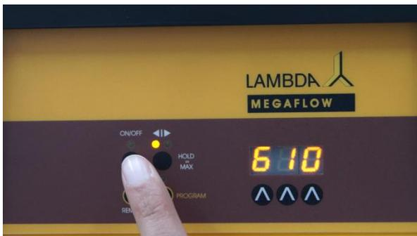
**Figure 1-1** Pressing **ON/OFF** button to switch **ON** the peristaltic pump
