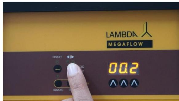
**Figure 2-8** By pressing the ◀▶ button, the time resolution can be set in minutes or 0.1 minutes. In the 0.1 minute time resolution a dot is displayed, e.g. “00.2”. The time resolution can be set individually for each program step.
