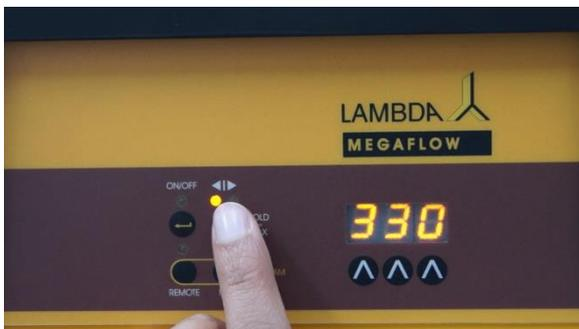
**Figure 1-5** LED illumination in the direction ◀| represents the clockwise rotation.
