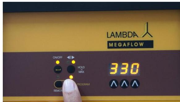
**Figure 2-20** To start the program, press the **RUN** button. The **RUN** and **ON/OFF** LEDs are on. To stop the running program definitively, press the **RUN** button. The **RUN** and **ON/OFF** LEDs are off
