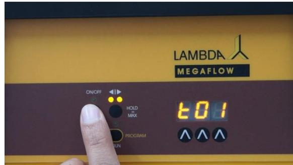
**Figure 2-6** Press the **ON/OFF** button. The indication “t01” will appear for a few seconds on the display indicating that the time period of the first step in minutes, can be programmed.
