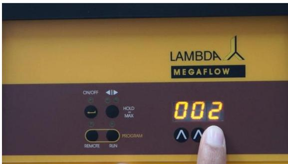
**Figure 2-7** Select the desired time period for the first program step by pressing the buttons ▲▲ below the display (from 0 to 999 minutes or 00.0 to 99.9 minutes).
