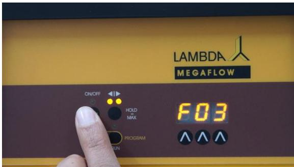
**Figure 2-15** After having entered the time of the last step, press the ON/OFF button.
